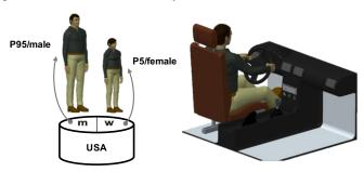
Fig. 2. Scaling of anthropometric human models (left); Anthropometric human model positioned in a car interior (right)
