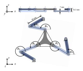
Fig. 5. Parameterized CAD model of 3RRR manipulator in initial configuration.
