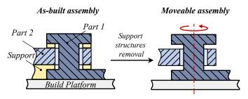
Fig. 1. Additive Manufacturing of non-assembly mechanisms by FDM using the example of a revolute joint.
