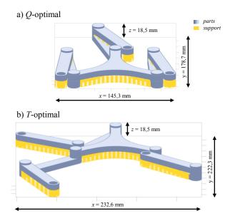
Fig. 6. Optimized variants of the 3RRR manipulator: a) for the support material quantity Q, b) for build time T.
