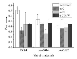
**Figure 2:** Mean friction coefficient  $\mu_{\text{rod}}$  of DLC coating samples (n = 3) against diverse sheet materials for sliding distance of 2.5 to 10 m
