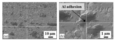
**Figure 8:** (a) Aluminium adhesions on the worn a-C:H:W coated surface and (b) adhesions caught by sharp edges of the flattened a-C:H:W grains taken from sample No. 36
