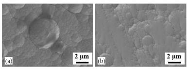
Figure 7: (a) Original and (b) polished a-C:H:W coated surface
