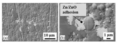
**Figure 9:** (a) Fe adhesions on the worn a-C:H:W surface and (b) adhesions trapped between valleys around polished particle grains taken from sample No. 32
