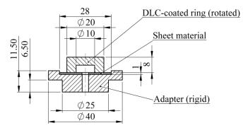
Figure 1: Cross section of the ring-on-disc-tribometer
