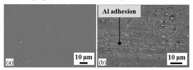
**Figure 4:** (a) ta-C coated surface before testing and aluminium adhesions on the worn ta-C coated surface taken from sample No. 16
