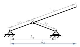
Figure 2 Example of a 2D skeleton model with dimensional tolerances
