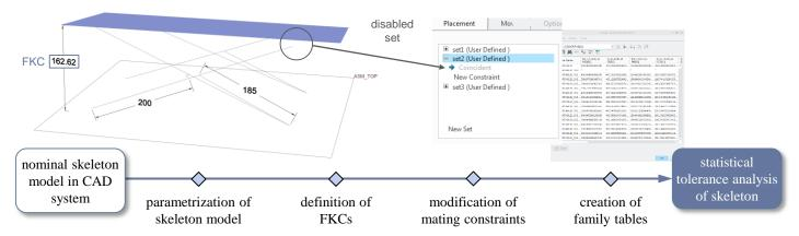
Figure 3 Process of the CAD-based tolerance analysis of skeleton models
