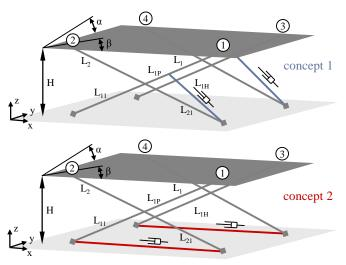
Figure 6 Skeleton model of a hydraulic scissor lift table for concept 1 (Figure 6a) and concept 2 (Figure 6b)
