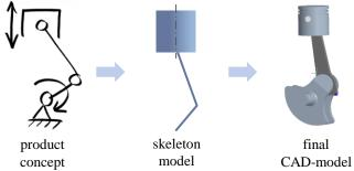
Figure 1 Different geometric degrees of details in product development, exemplary for a thrust crank drive
