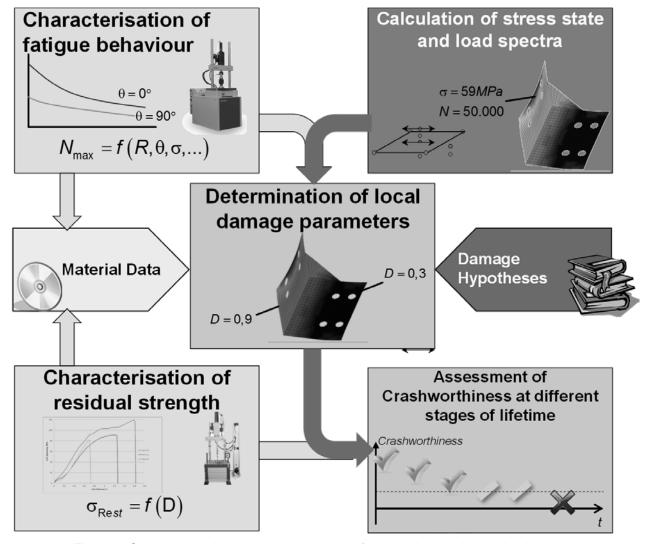
Figure 7. Steps required towards consideration of mechanical ageing in simulative crashworthiness evaluation
