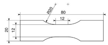
Figure 3. Test specimen according to Becker, 2009
