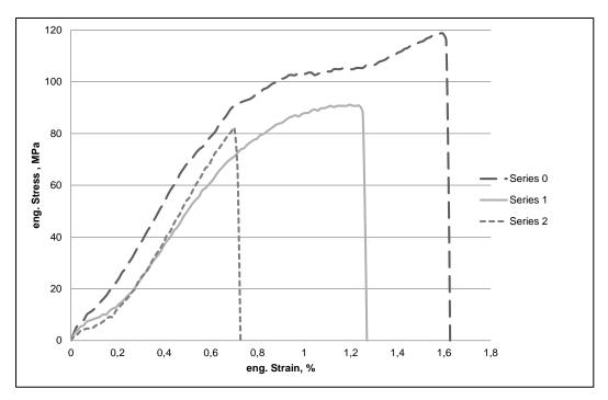
Figure 5. Stress-strain-diagrams (averaged) of the series 0, 1, and 2
