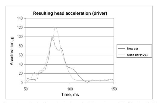
Figure 1. resulting head acceleration in used vehicle and new vehicle (Kamber, 2005)
