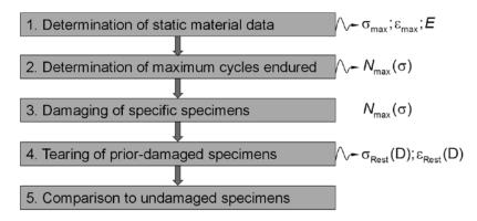
Figure 2. stepwise testing procedure
