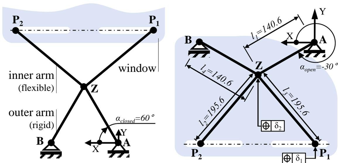
Figure 3. Cross-arm window regulator: (left) closed window (right) opened window
