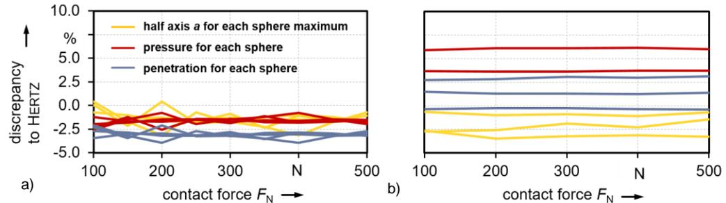
Figure 2: relative comparison of PinP to HERTZ of the area, pressure and penetration
