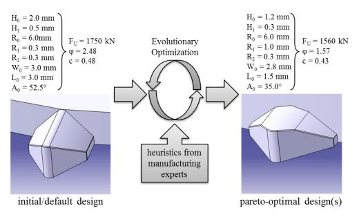
Figure 5: Initial and an optimized version of the locking teeth with according process parameters. Note, that there is mostly more than one pareto-optimal design.
