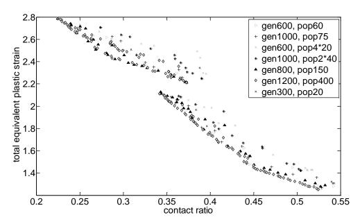
Figure 4: Pareto chart of plastic strain and contact ratio with different optimization configurations (pop= size of population, gen= number of generations).
