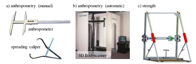
Figure 2. Examples of instruments to measure a) anthropometric data manually or b) automatically as well as c) the strength of the human body (DIN, 2017; Hotzman et al., 2011; Wakula et al., 2009)
