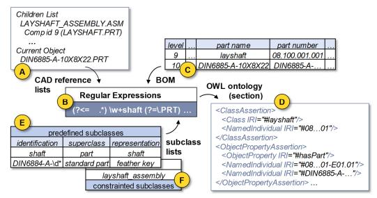
Figure 3. Automated generation of ontologies
