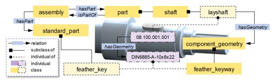
Figure 2. Example for an ontology-based product representation with pre-defined and generated (dashed boxes) classes, individuals and relations
